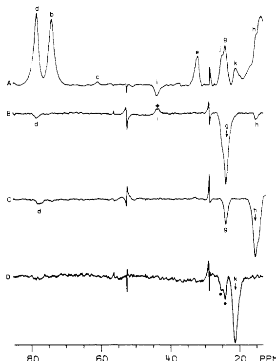
FIGURE 4: (A) Hyperfine-shifted portion of the 360-MHz ^1\text{H} NMR spectrum of 3 mM HRP-I in 99.8% ^2\text{H}_2\text{O} at 15 ^\circ\text{C} , pH 7.0. The spectrum was collected with a Redfield 2-1-4-1-2 pulse sequence with the spectral window optimized for the region 10–40 ppm. The downfield 40–80 ppm region is the second and third excitation windows of the pulse sequence, and the signals in this region have their intensity and phases according to the phase modulation of the Redfield pulse sequence (Redfield et al., 1975). Peak labeling is the same as in trace A of Figure 3. Note that peak i has opposite phase and peaks a, c, and f fall near the crossover point of the excitation windows, and hence, these resonances are not excited. (B–D) NOE difference spectra generated as described in Figure 1. The downward arrow shows the peak being saturated; a filled circle (●) denotes off-resonance effects, and (◆) signifies NOEs from off-resonance saturated peaks. (B) Saturation of peak g yielding NOEs to peaks h and d; note the NOE to peak i from the partial saturation of peak j. (C) Saturate peak h at 15.4 ppm; note the large reciprocal NOE to peak g and a weak NOE to 8- \text{CH}_3 . (D) Saturation of peak k showing the absence of any NOE to the resolved signals.
